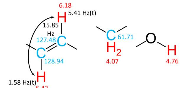
Both proton multipletts have a common coupling constant of **15.85 Hz** (averaged value). Thus the protons are trans to each other.
